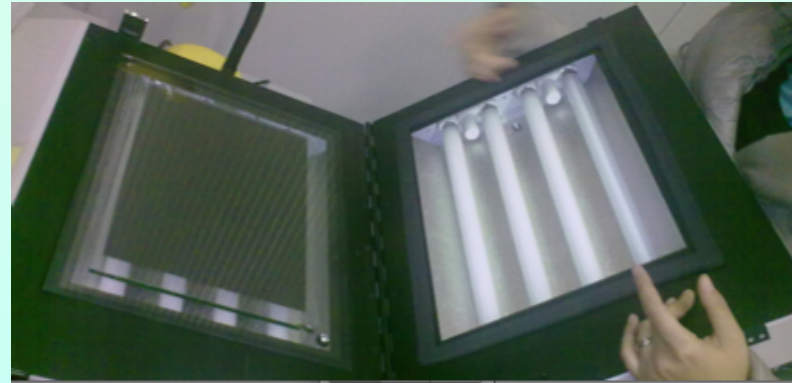
photoresist masking and UV exposure
