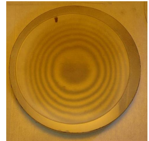
Fringes between mould and glass very circular and without dust contamination
