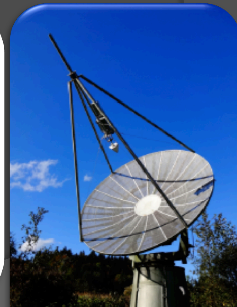
FIG. 2.— Image of the 5m radio dish at the Bleien Observatory. From the image one can see the wire meshed reflector, as well as the four struts which hold the horn receiver in focus.
